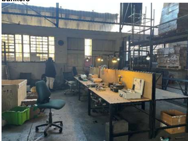
Photo 5: E-waste Dismantling stations
