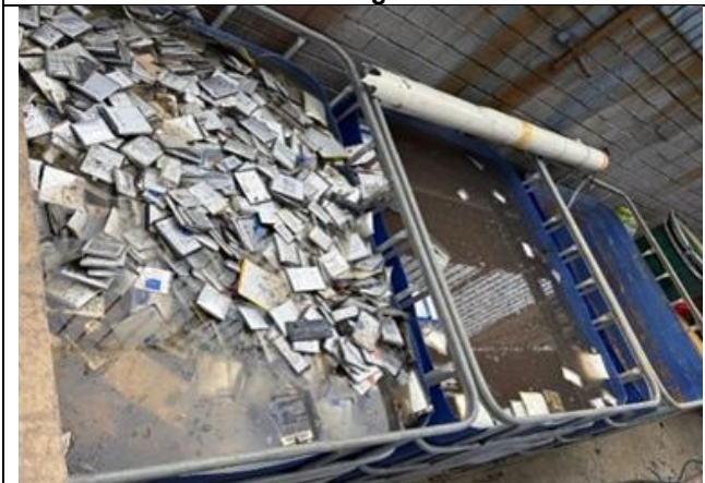
Photo 7: LIB Discharge Area
