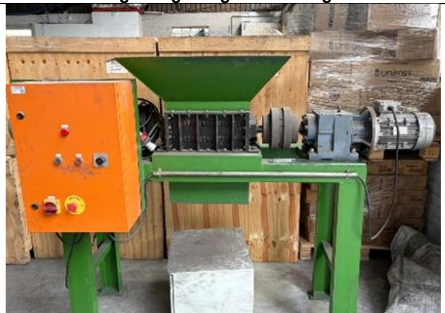
Photo 8: LIB Shredder Station
